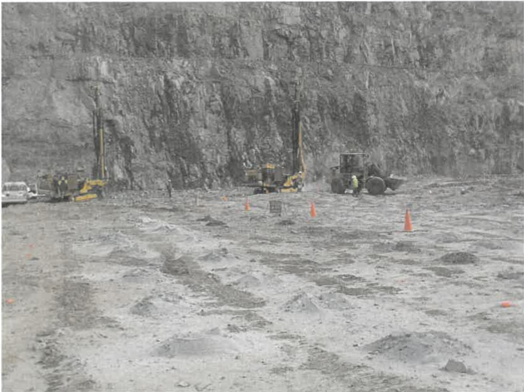
Blast holes being drilled in Nolan's Pit (August 2001)
