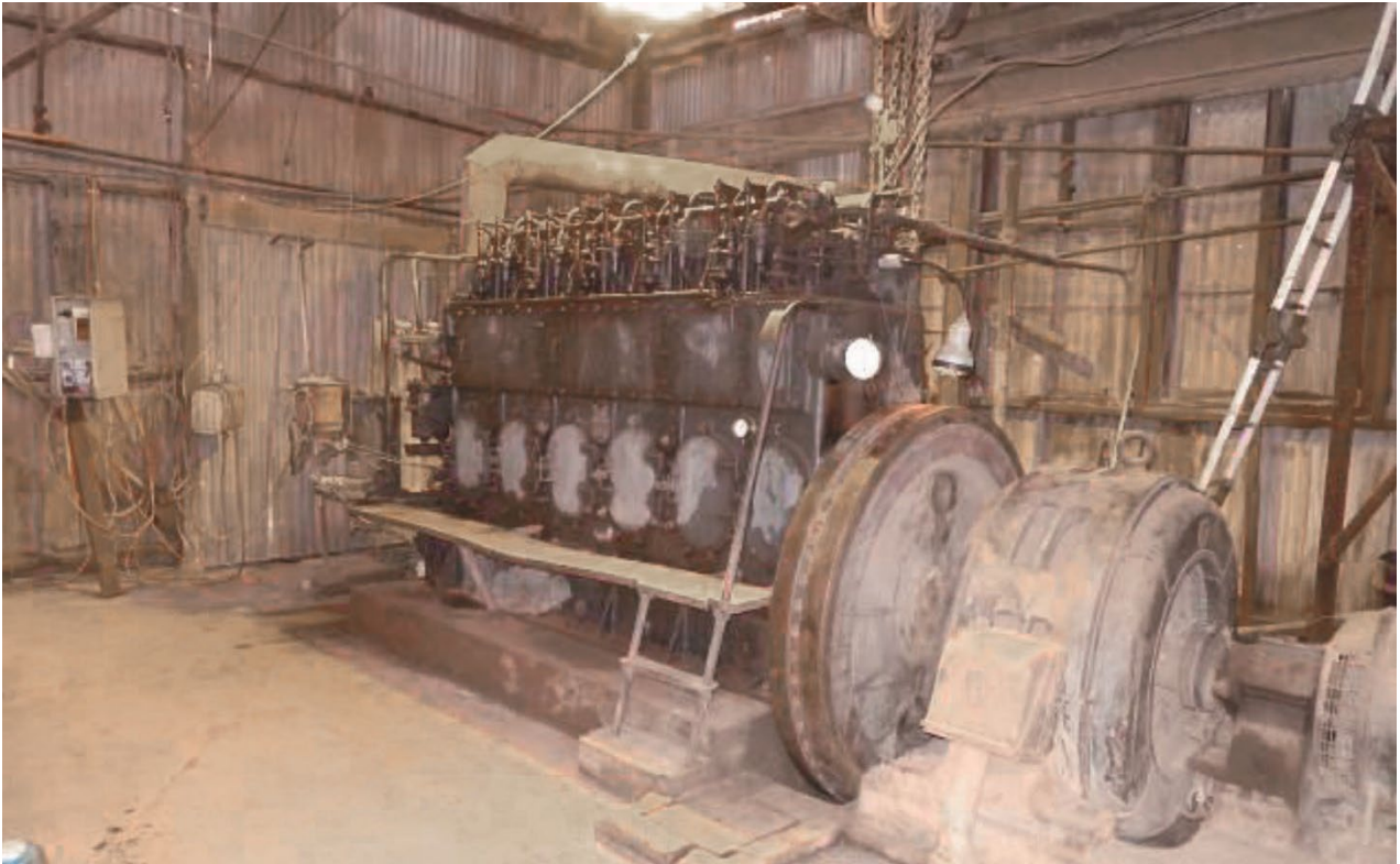
Figure 19: Comet Gold Mine Ruston Diesel Power Engine.
