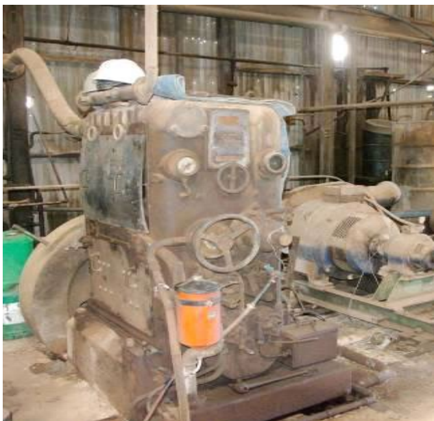
Figures 18(a) & 18(b): Comet Gold Mine Blackstone Diesel Power Engine.
