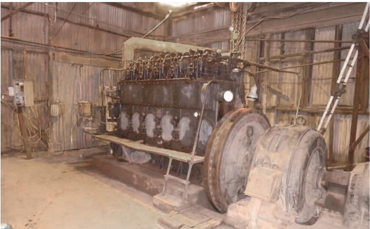
Figure 22: Comet Gold Mine Ruston Diesel Power Engine
