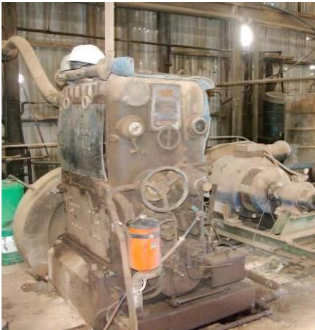
Figures 21(a) & 21(b): Comet Gold Mine Blackstone Diesel Power Engine
