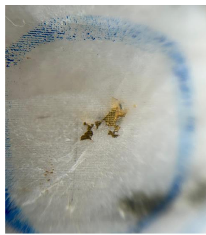
Figure 5d: Visible gold in 24BTDD002, associated with galena (left), free gold (right).
