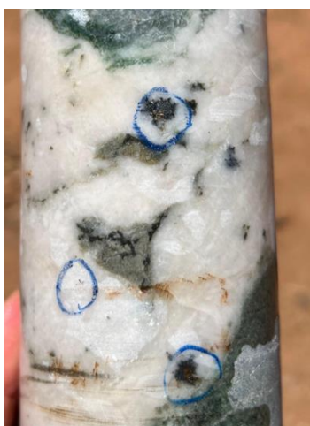
Figure 5c: Visible gold in 24BTDD002, (blue circle) associated with galena.
