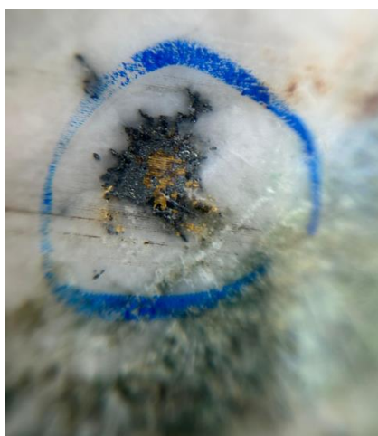
Figure 5d: Visible gold in 24BTDD002, associated with galena (left), free gold (right).
