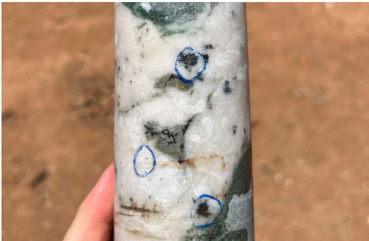
Figure 4: Visible gold in 24BTDD002 (circled in blue) associated with galena
