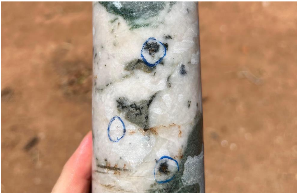
Figure 1: Visible gold in 24BTDD002 (circled in blue) associated with galena
