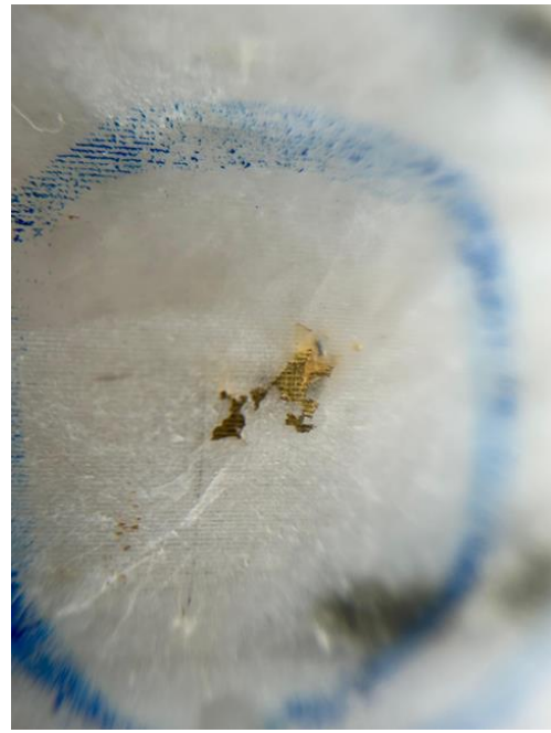
Figure 2: Close up of visible gold in 24BTDD002. Close association with galena visible (left), free gold (right)
