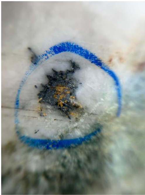
Figure 2: Close up of visible gold in 24BTDD002. Close association with galena visible (left), free gold (right)
