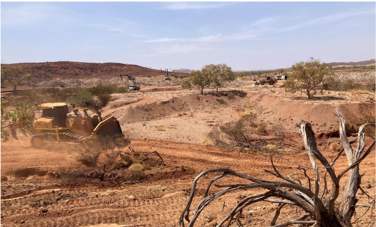
Figure 2: Clearing of Blue Bar waste dumps, with stockpiles in background and laydown yard
