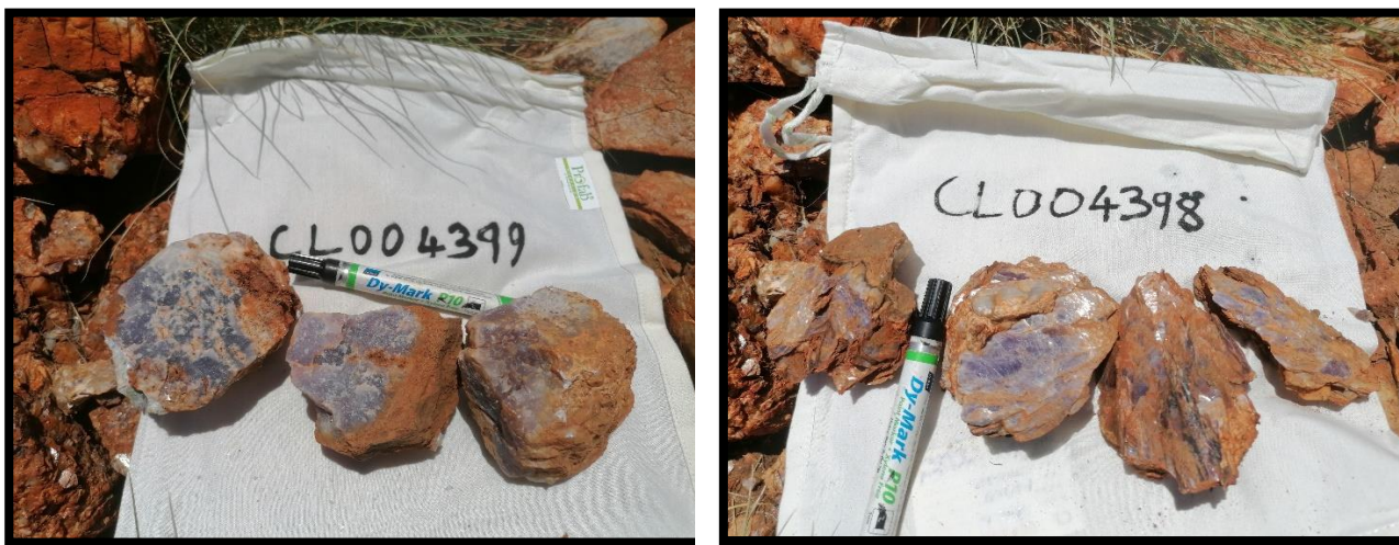
Figure 4 – Samples of coarse spodumene (LHS) and coarse lepidolite (RHS) from samples sent for assay.
