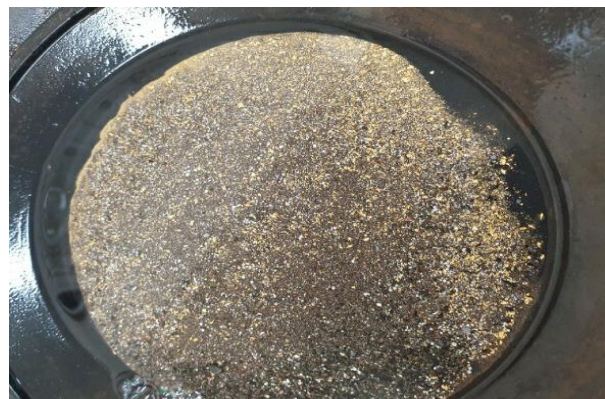
Figures 1-4: Just-in-Time gravity gold recovered from the Knelson concentrator
