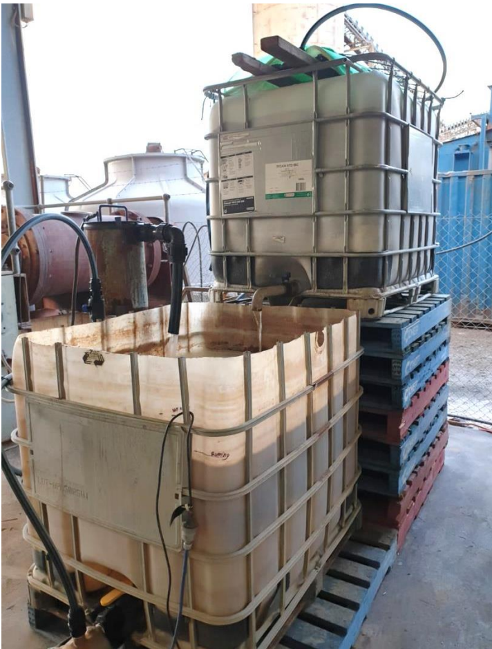
Figure 1: Vat Leach Trial processing 1.425t of '+180 microns to -3mm' ore from Bamboo Creek Vat
