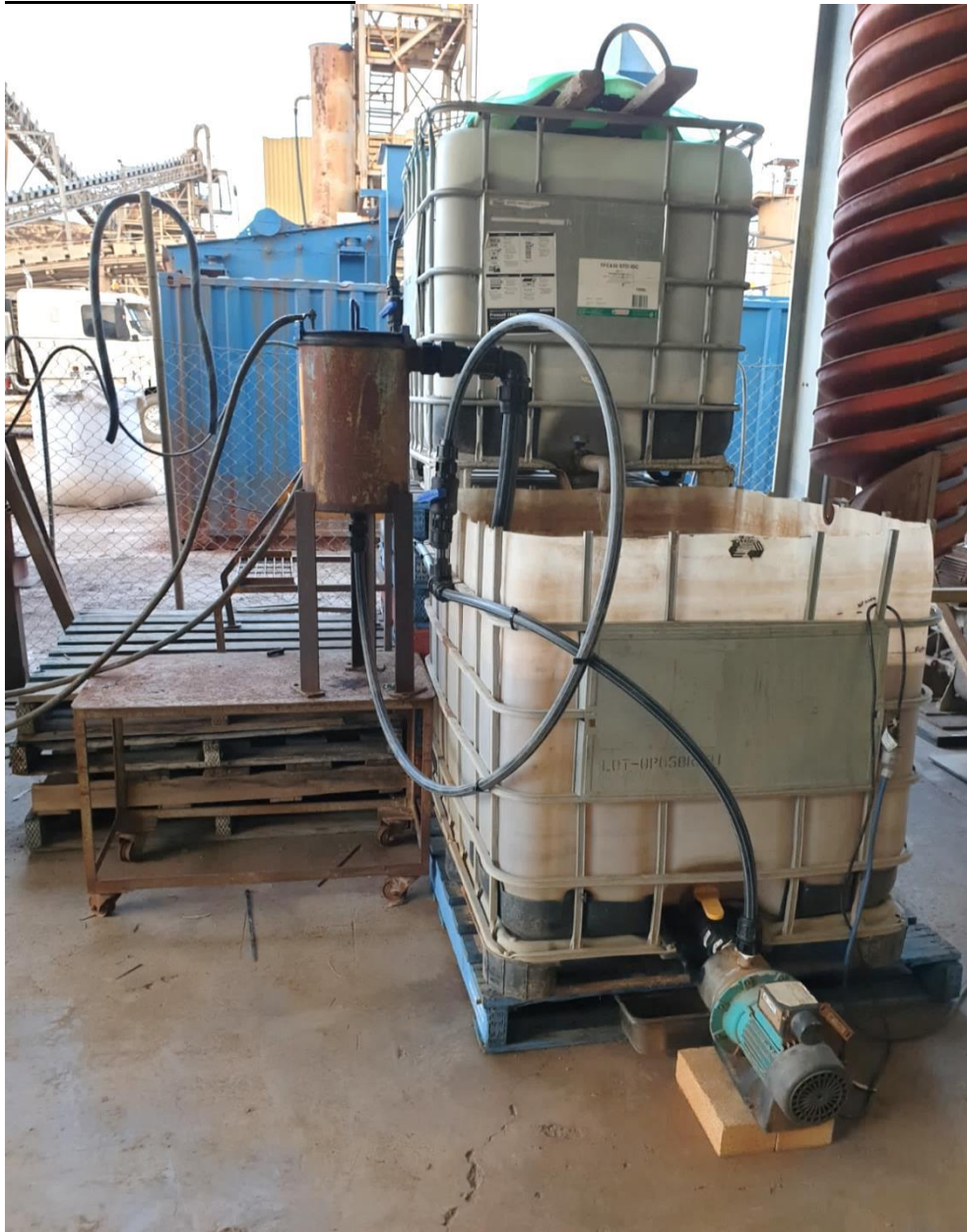
Figure 5: Vat Leach Trial processing 1.425t of '+180 microns to -3mm' ore from Bamboo Creek Vat
