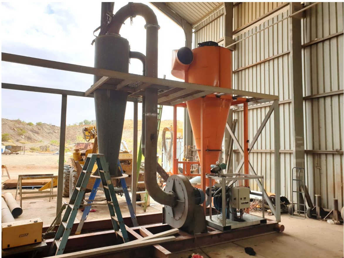
Figure 3:Part of Haoma’s ‘special equipment’ designed and being constructed to recover 29.32g/t gold.
