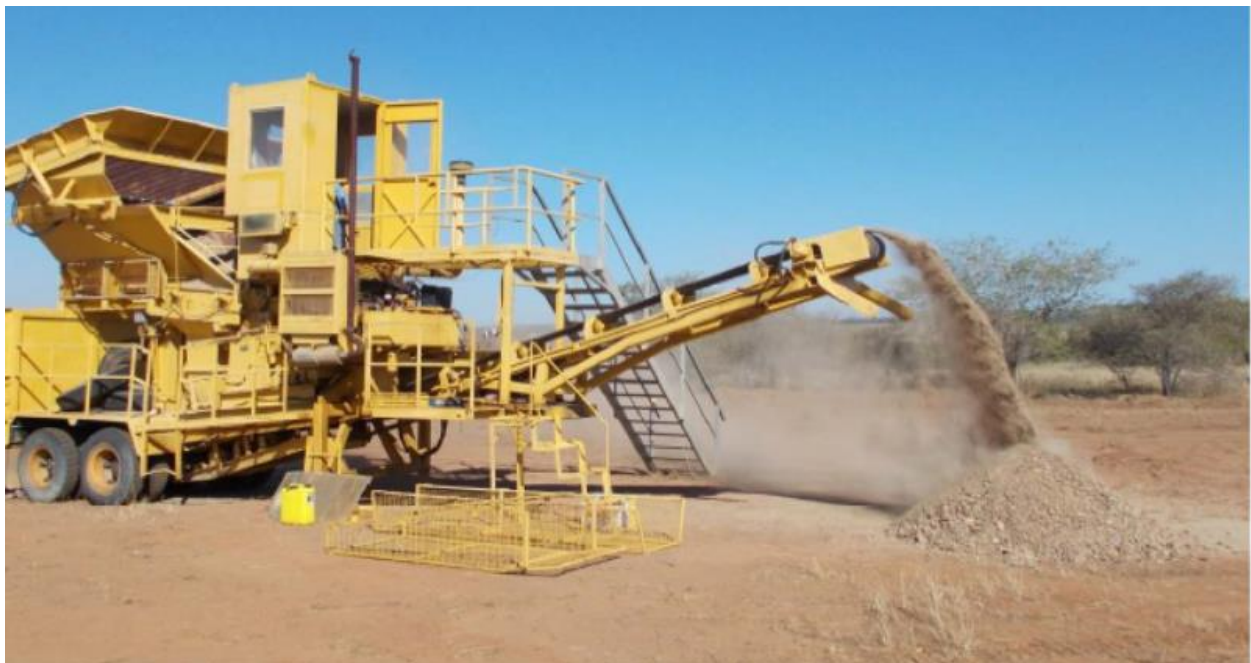
Figure 15: Haoma's Ravenswood Mobile Crusher being tested during commissioning at Copper Knob (ML1330)
