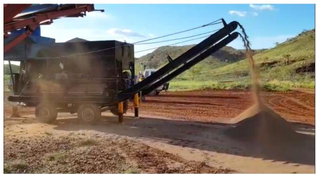
Figure 2: Dry Blower being tested in Nuggety Gully at Bamboo Creek.
