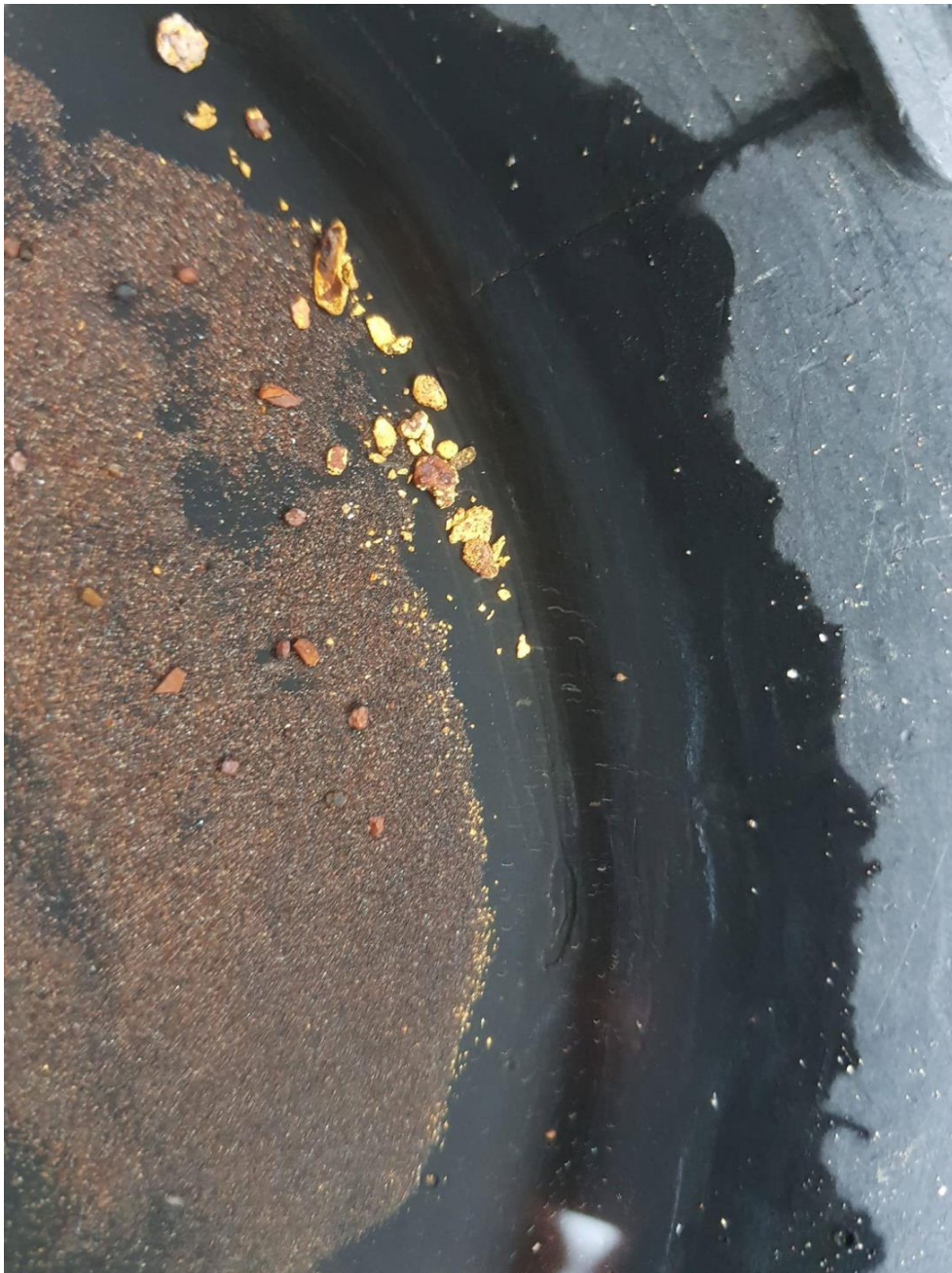
Figure 3: 2.2 grams of gold recovered by gravity separating a one tonne bulk sample of area C2 Conglomerate Ore. The sample involved only an initial stage of coarse crushing.
