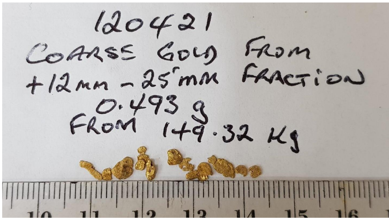
Figure 4b: Gold nuggets recovered by gravity after milling the +12mm -25mm fraction of the 1.4 tonne sample of Conglomerate Ore.
