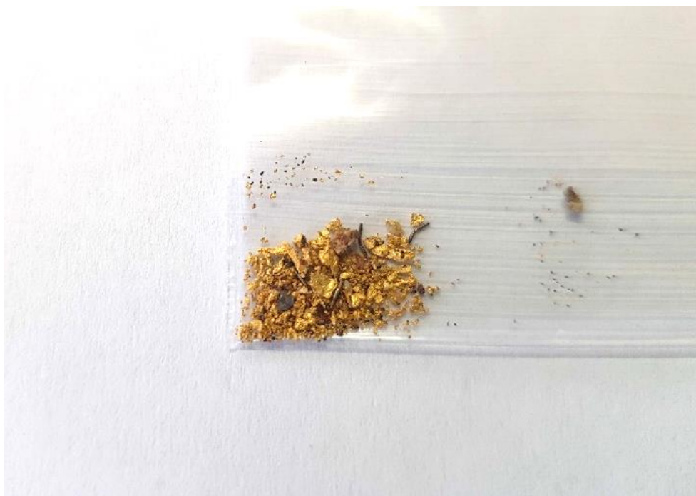
Figure 12: 'Fine' gold collected from area C2 Conglomerate Formations to the South West of the Comet Mine, total sample weight 0.183g.
