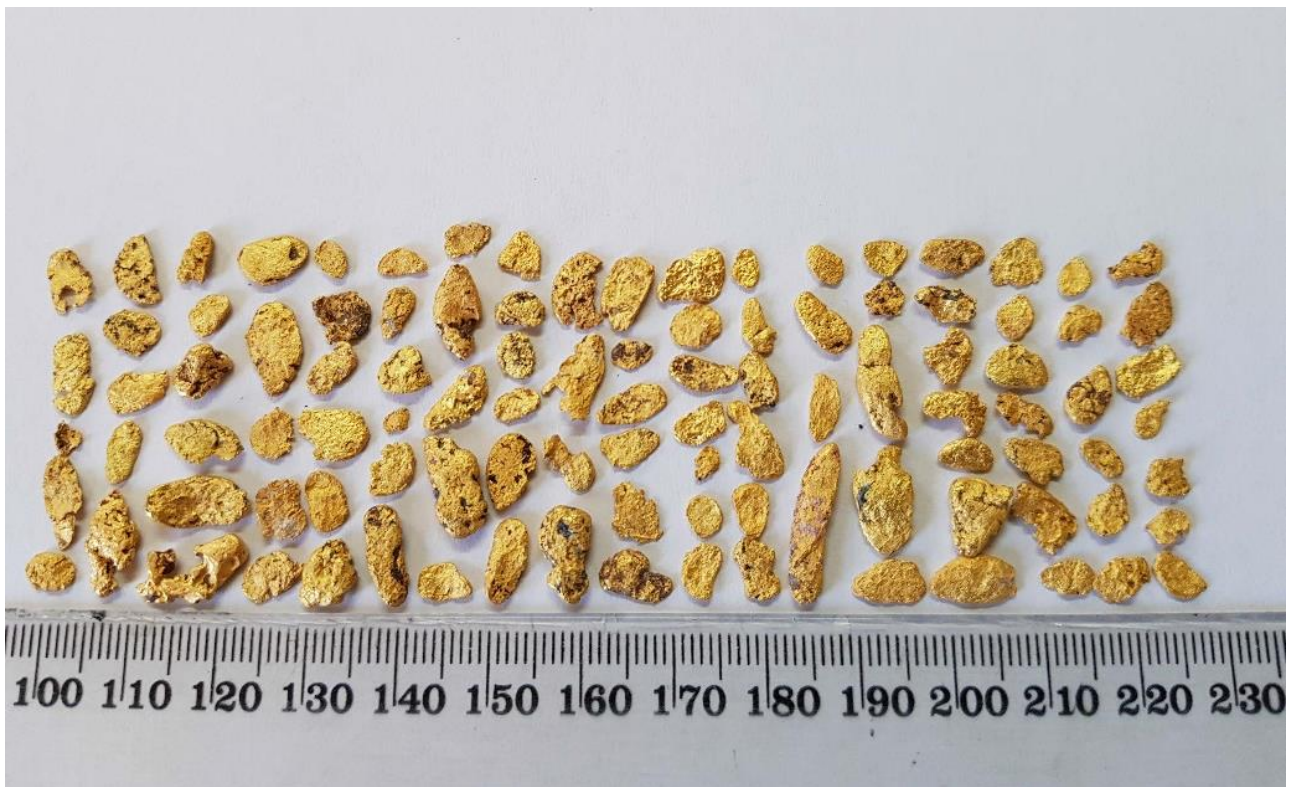
Figure 11: Nuggets collected from area C2 Conglomerate Formations to the South West of the Comet Mine, total weight of nuggets 33.167g.
