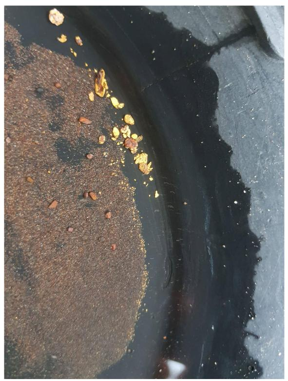
2.2 grams of gold recovered by gravity separation after initial stage of coarse crushing a one tonne bulk sample of area 'C2' conglomerate material
