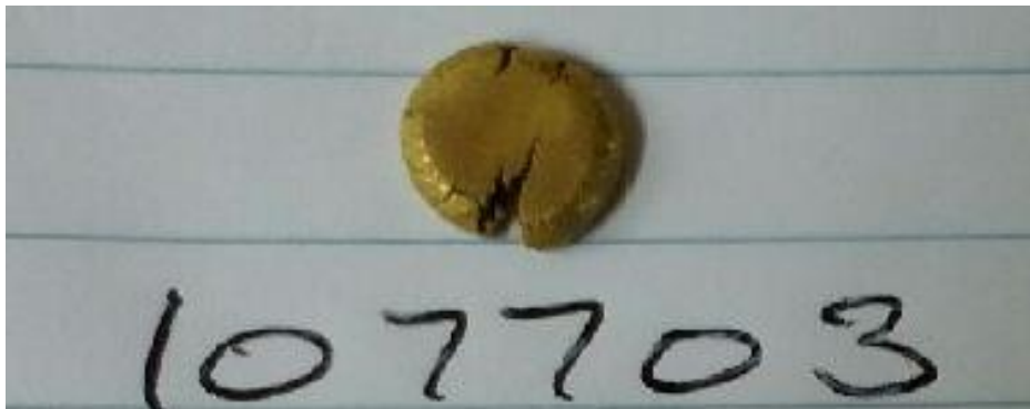
Figure 1: 2.714g gold button recovered from 361g sample of ‘Gold Concentrate’
