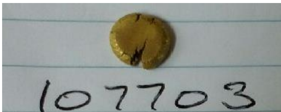
Figure 2: 2.714g gold button recovered from 361g sample of 'Gold Concentrate'
