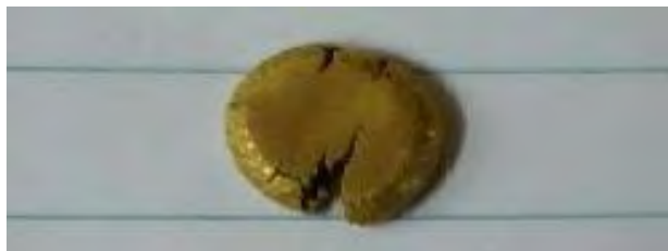
Figure 3: 2.714g gold button recovered from 361g sample of 'Gold Concentrate'
