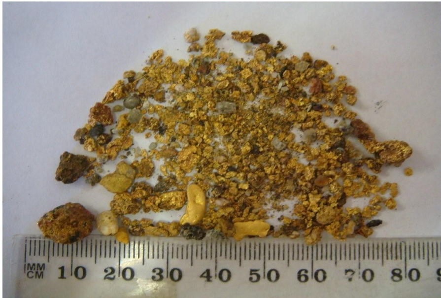
Coarse 'gravity' gold from Bamboo Creek Tenements
