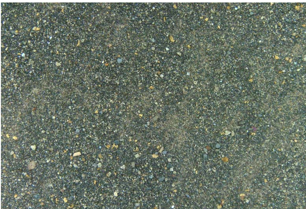
Close-up showing 'free' gold in gravity 'concentrate' from Bamboo Creek Tenements
