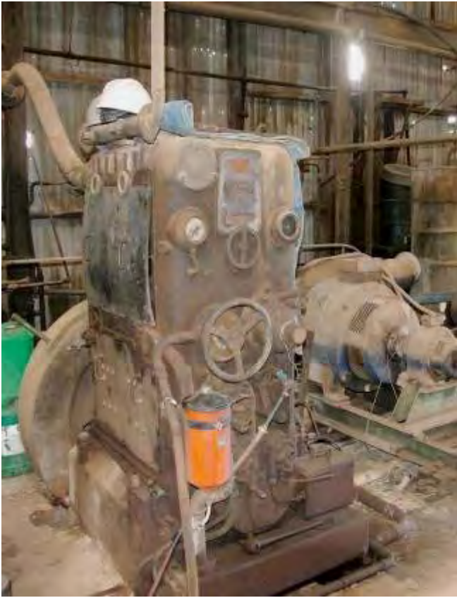
Figures 14 & 15: Comet Gold Mine restored Blackstone Diesel Power Engine
