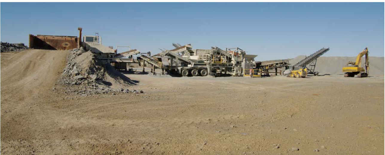
Figure 14: BGC Contracting Pty Ltd Portable Crushing Plant at Cookes Hill Dolerite Quarry
