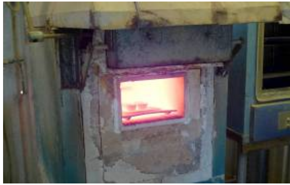
Figure 3(d): Bamboo Creek Muffle Furnace
