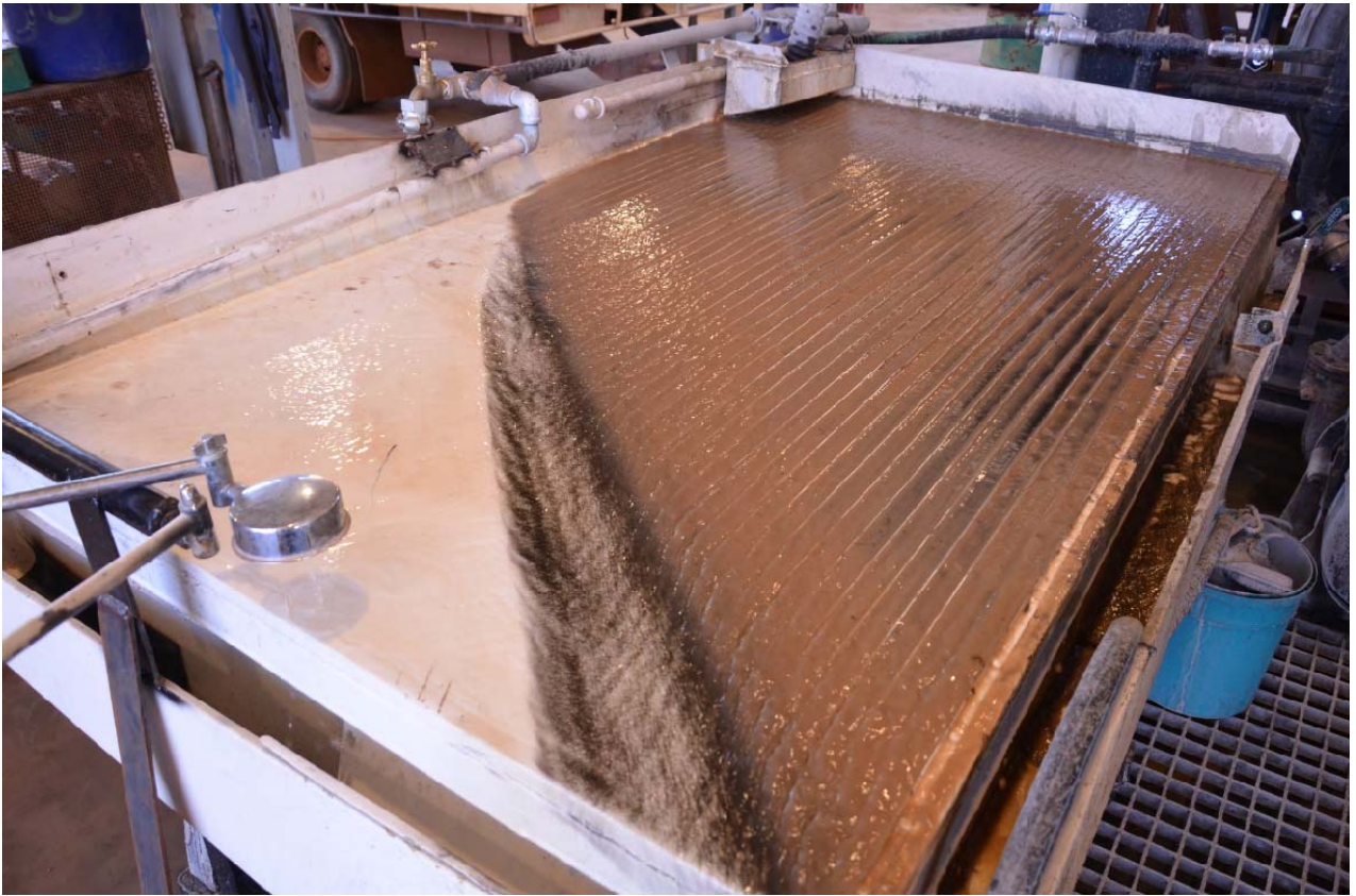
Figure 13b: Polymetallic ore being concentrated by Wilfrey Gravity Table
