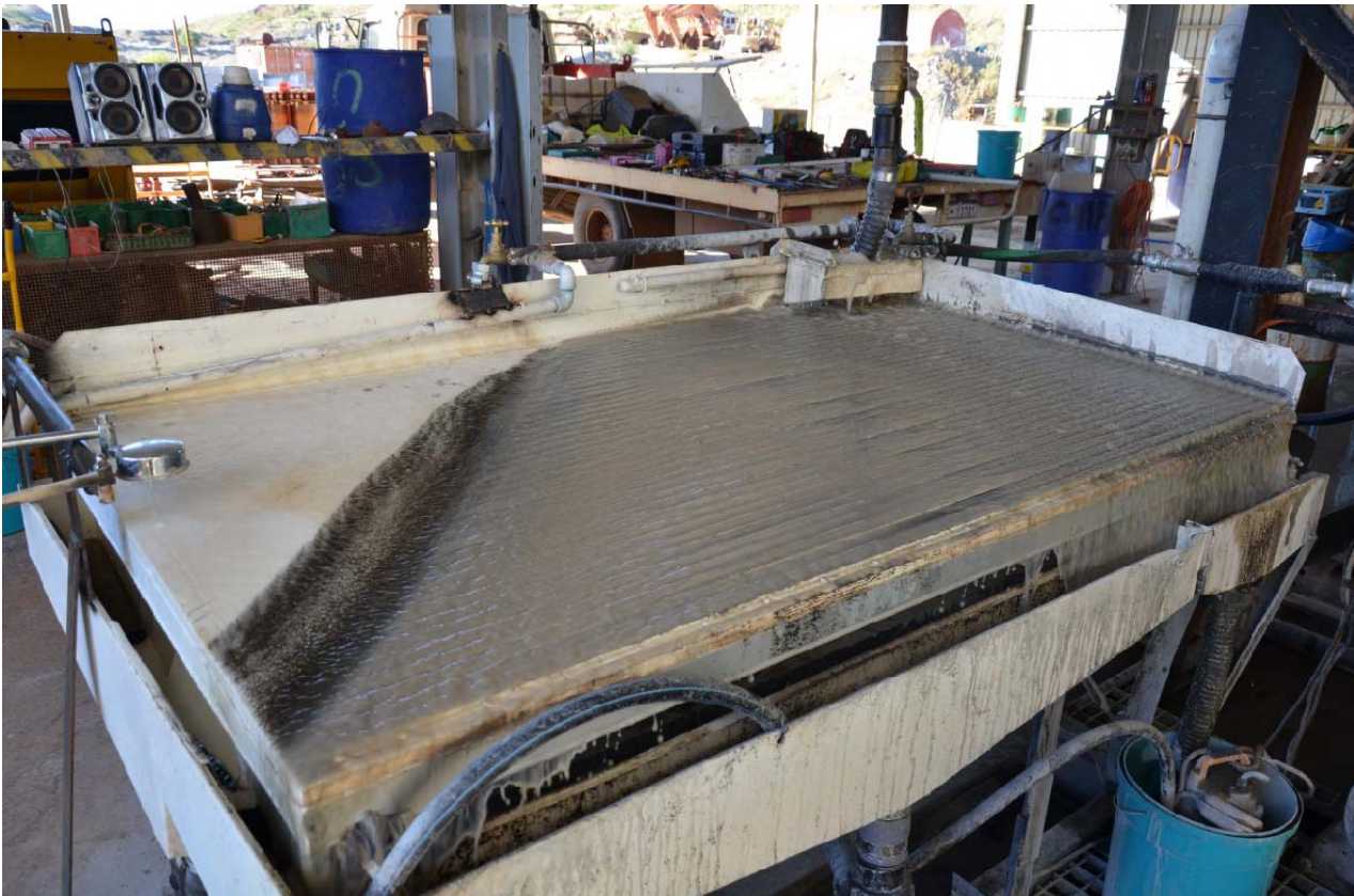
Figure 13a: Wilfrey Gravity Table used to collect a Polymetallic ore ‘concentrate’
