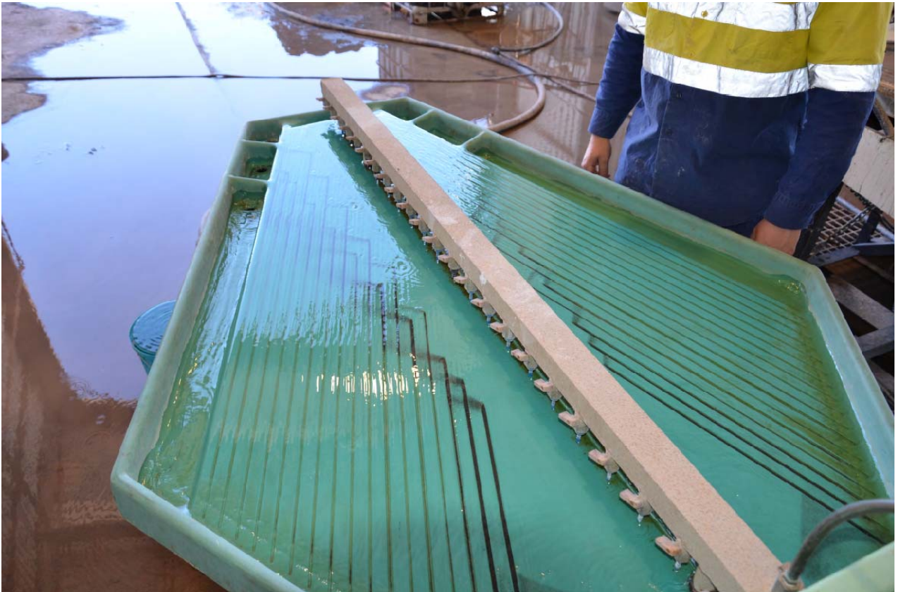
Figure 14: Polymetallic ore being concentrated and collected by Gemeni Gravity Table
