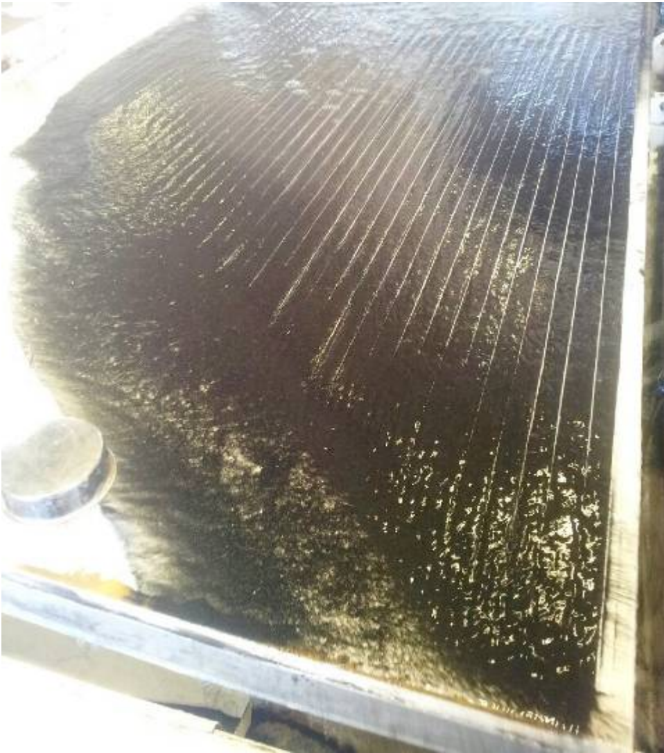
Figure 13c. The left side of the Wilfrey Gravity Table shows polymetallic ore
