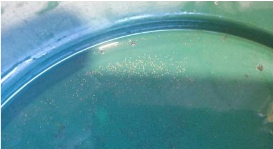
Figure 15. Polymetallic ore fragments shown with the use of a panning dish.
