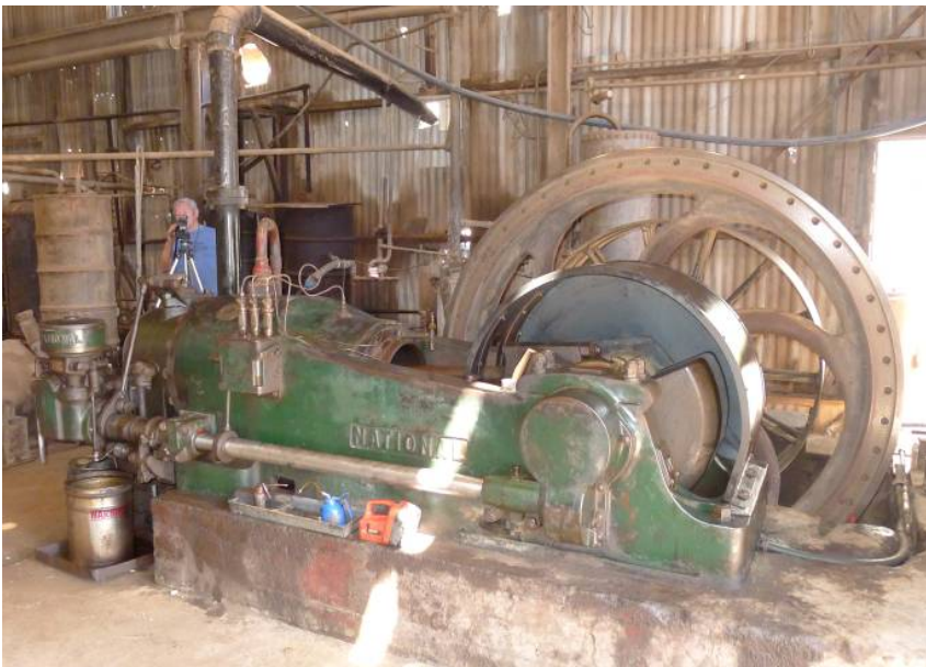
Figure 14: Restored National Diesel Power Engine
