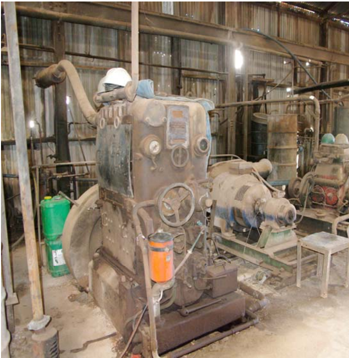
Figures 21 – 23: Comet Gold Mine Historic Diesel Power Station showing Blackstone Engine which has recently been restored
