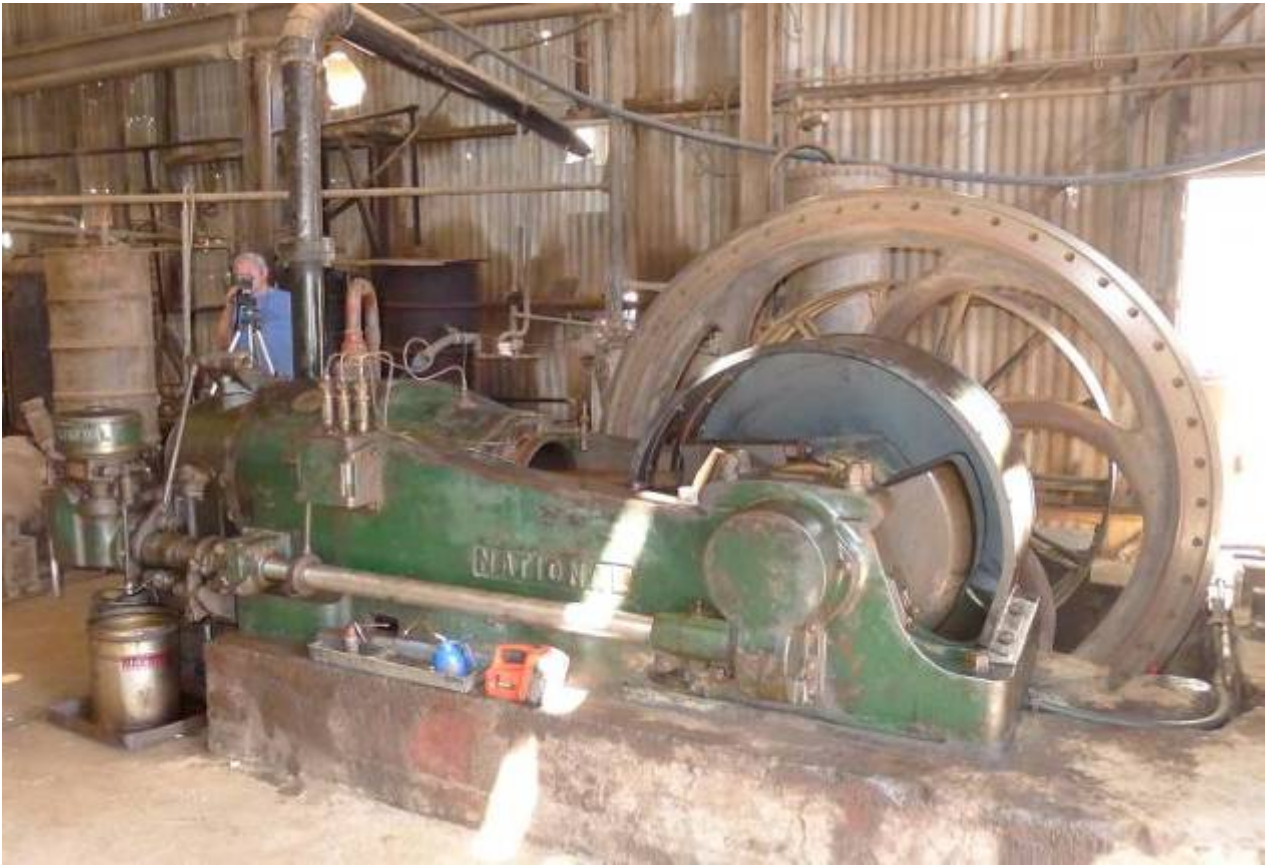
Figure 17: Comet Gold Mine restored Blackstone Diesel Power Engine
