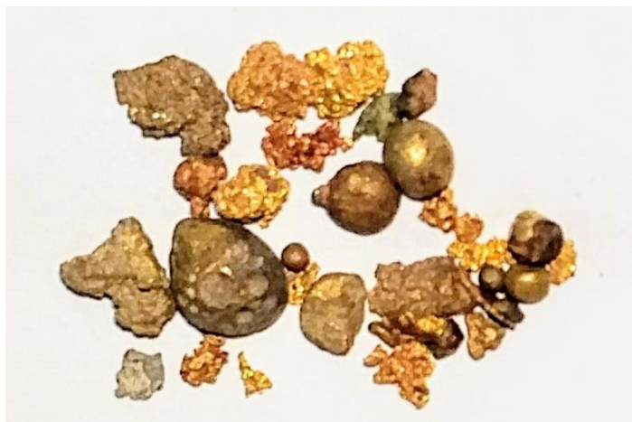
Figure 2d: Free gold recovered from gravity circuit.
