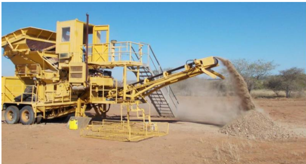
Figure 17: Haoma’s Ravenswood Mobile Crusher being tested during commissioning at Copper Knob (ML1330)
