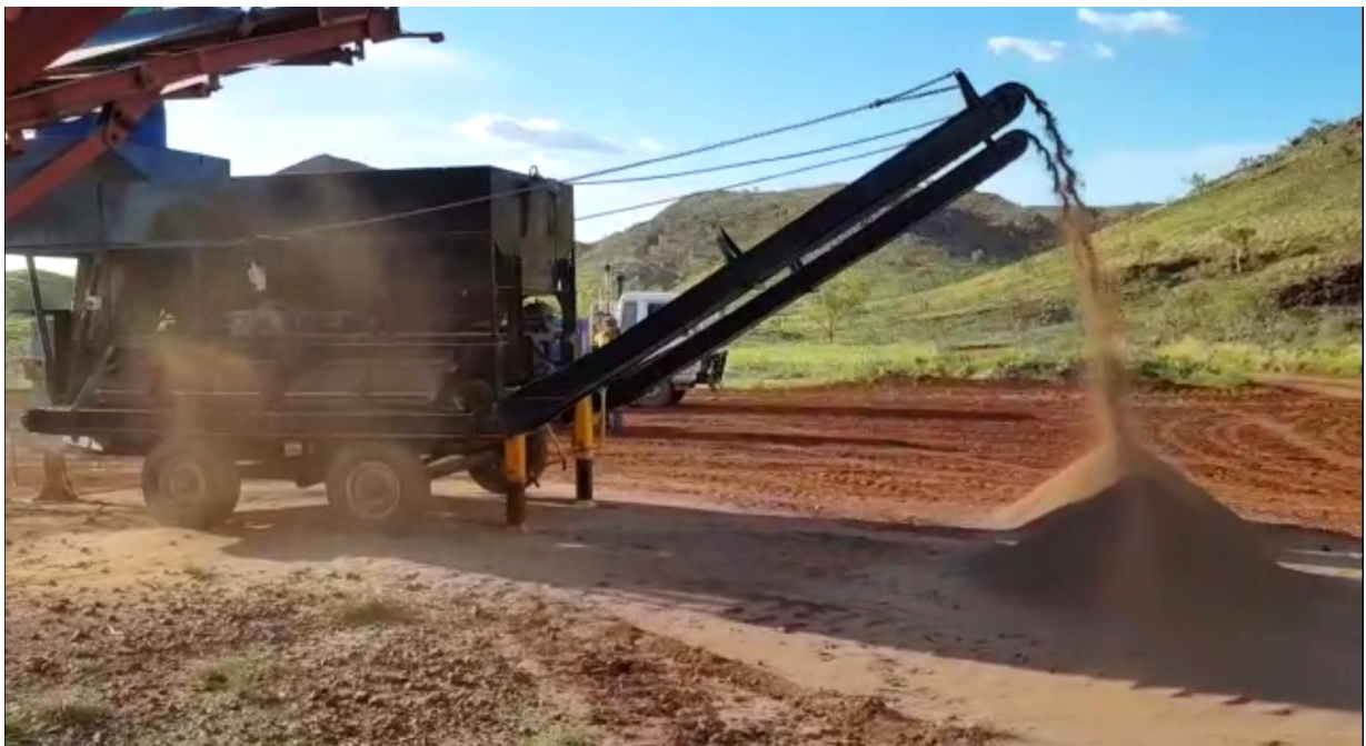
Figure 2b: Screening Plant and Dry Blower being tested in Nuggety Gully at Bamboo Creek.
