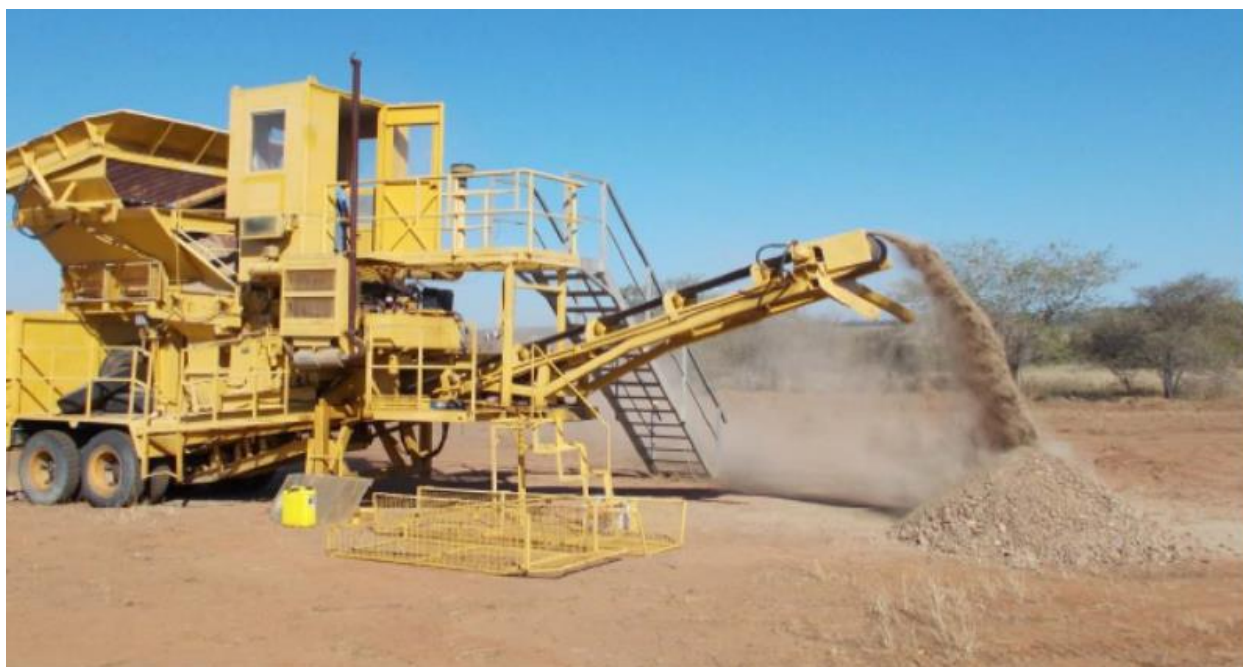
Figure 15: Haoma's Ravenswood Mobile Crusher being tested during commissioning at Copper Knob (ML1330)
