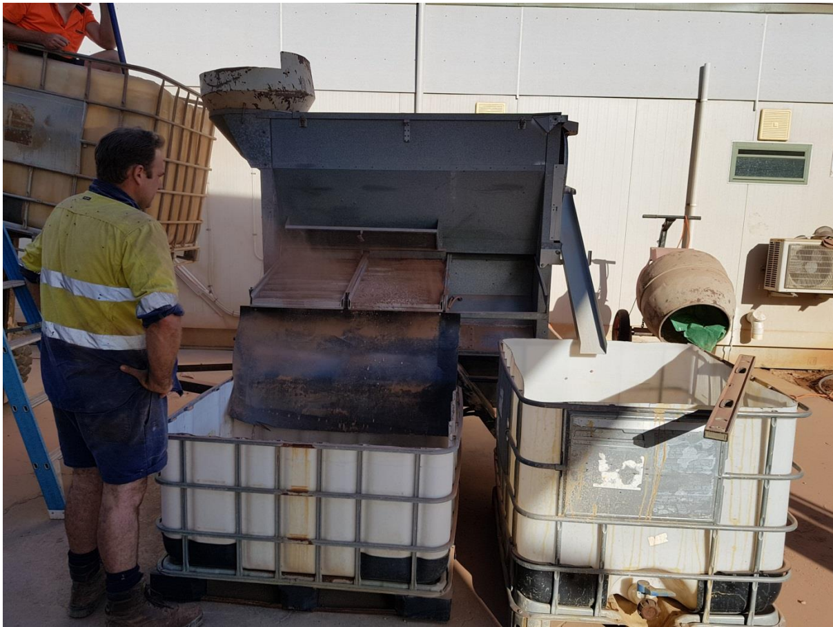
Figure 9: ‘Dry blower’ processing Just-in-Time conglomerate bulk ‘Channel sample’. (Trial 1208)
