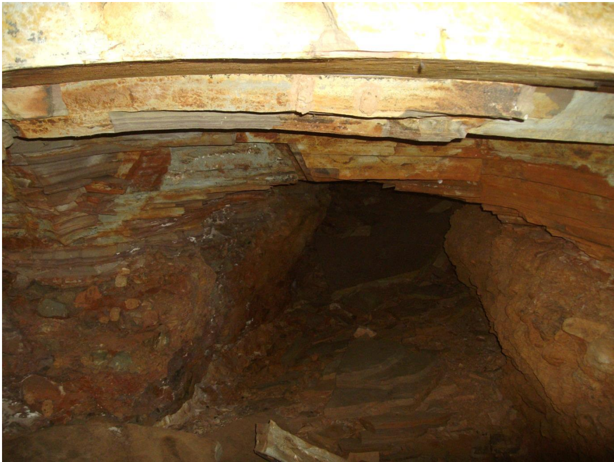
Figure 5: Ferruginous auriferous conglomerate exposed in Just-in-Time adit, showing sharp contact with planar bedded sandstone in the hanging-wall. The conglomerate is approximately 0.8m wide (true width) where intersected with the sandstone. The adit entrance is located at 21-15-058S, 119-43-266E, it is 24m long and horizontal.
