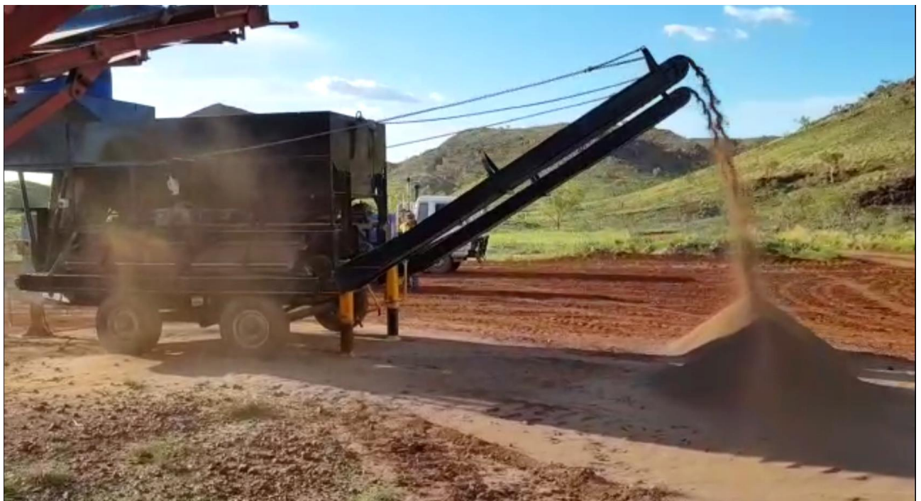
Figure 6: Dry Blower being tested in Nuggety Gully at Bamboo Creek.
