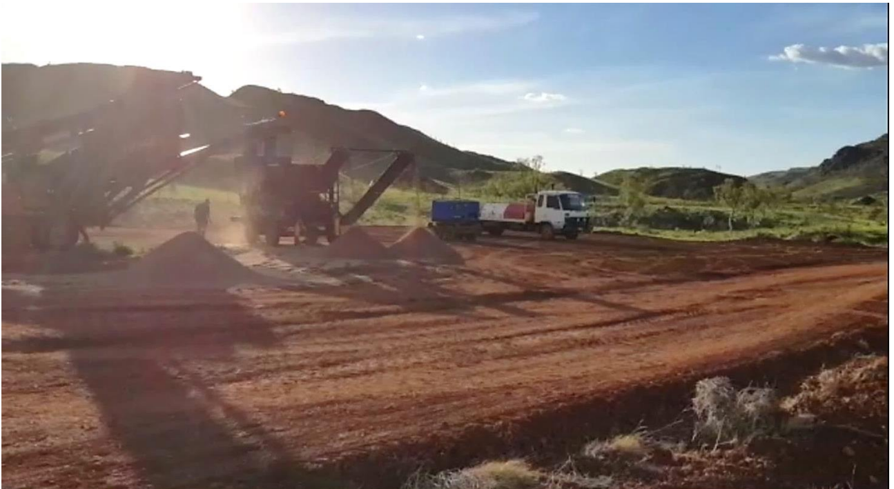
Figure 5: Screening Plant and Dry Blower being tested in Nuggety Gully at Bamboo Creek.
